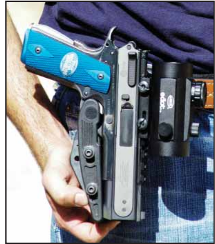
Weird gear: Neil Hogue shot with Hogue Inc.'s custom upper for the 1911. The slide doesn't reciprocate. Instead, a relatively small bolt inside the slide does all the work. Note the stylish Steel Challenge grip panels.
